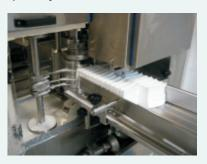
The active solution will be transported to the machine where the tissue material will be completely impregnated. The wet tissues are folded and cut automatically.
