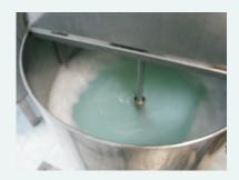
After demineralizing and sterilizing the water the formula for the specific application will be prepared. The special treating of the water is necessary to keep the content completely free from bacterials.
